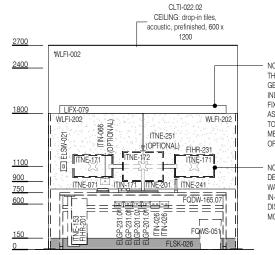
NOTE: LIGHTING FIXTURES ARE INDICATIVE. THE OVERALL COMBINATION OF DIMMABLE GENERAL ROOM LIGHTING, DIMMABLE INDIRECT LIGHTING (WALL AND/OR CEILING FIXTURES), AND THE USE OF FFE ITEMS SUCH AS BACK LIT MONITORS AND KEYBOARDS IS TO BE ASSESSED TO ENSURE THE SPACE. MEETS REQUIREMENTS FOR PERFORMANCE OF REVIEWING AND REPORTING TASKS
