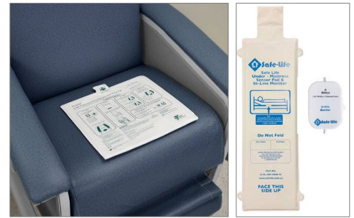
Figure 79 Examples of falls prevention devices such as chair pressure pads and under-mattress pressure pads, that may be connected to an outlet on a nurse call button face plate to trigger an alert to staff when a patient who is at risk of falls is exiting a bed/ chair
