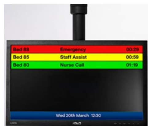
Figure 82 Example of a ceiling mounted LCD nurse call annunciator display screen
