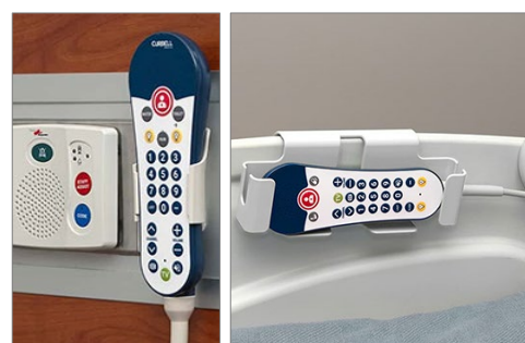
Figure 74 Examples of patient handsets with light control and patient entertainment system controls, and speakers in holders a) clipped to side rails of a patient bed, and b) mounted on a medical services panel
