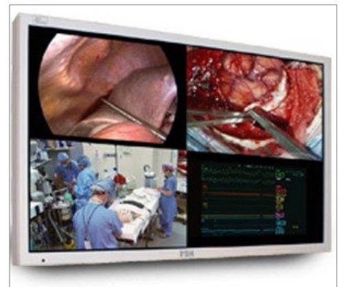
Figure 100 Example of a surgical display screen with four inputs displayed (from laparoscopic camera, operating light integral camera, in room camera, patient monitor)
