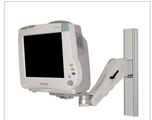
Figure 93 Example of a patient monitor on an articulated arm attached to a wall bracket
