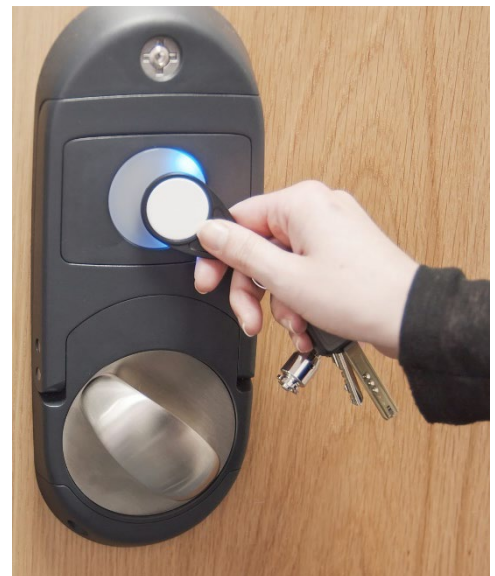
Figure 91 Example of anti-ligature door handle with electronic access control with override
